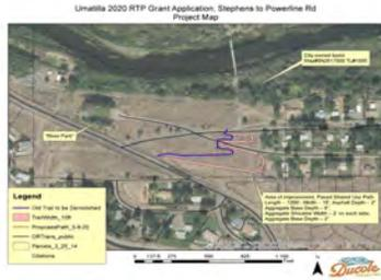
**Project Scope:** Planning, design, and construction of a section of path that will connect the South Hill region to the west side of the pedestrian bridge, and ultimately to the downtown area. The new ADA-compliant paved path will be approximately 1,000 feet in length running from Powerline Road to Stephens Avenue to connect to the reconstructed footbridge discussed later in the packet. The project will also include demolishing and removing the existing substandard asphalt path.
